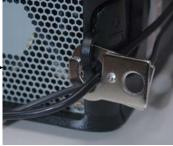
Steel cable trap captures and secures Dell CPU, internal components, mouse and keyboard cables.
