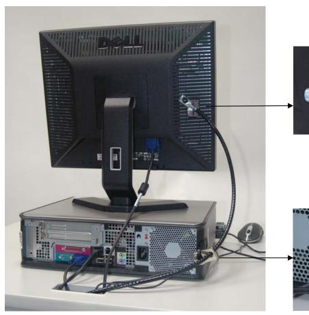
Special flat panel monitor anti-theft brackets slide easily into vent slots on back of monitor.
